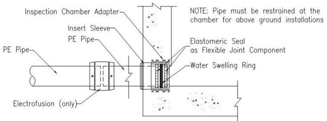
Type A – Typical flexible connection for a PE Pipe to concrete Manhole Chamber
