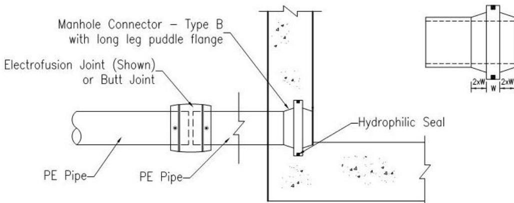
Type B – Typical rigid connection for PE Pipe to concrete Manhole Chamber
